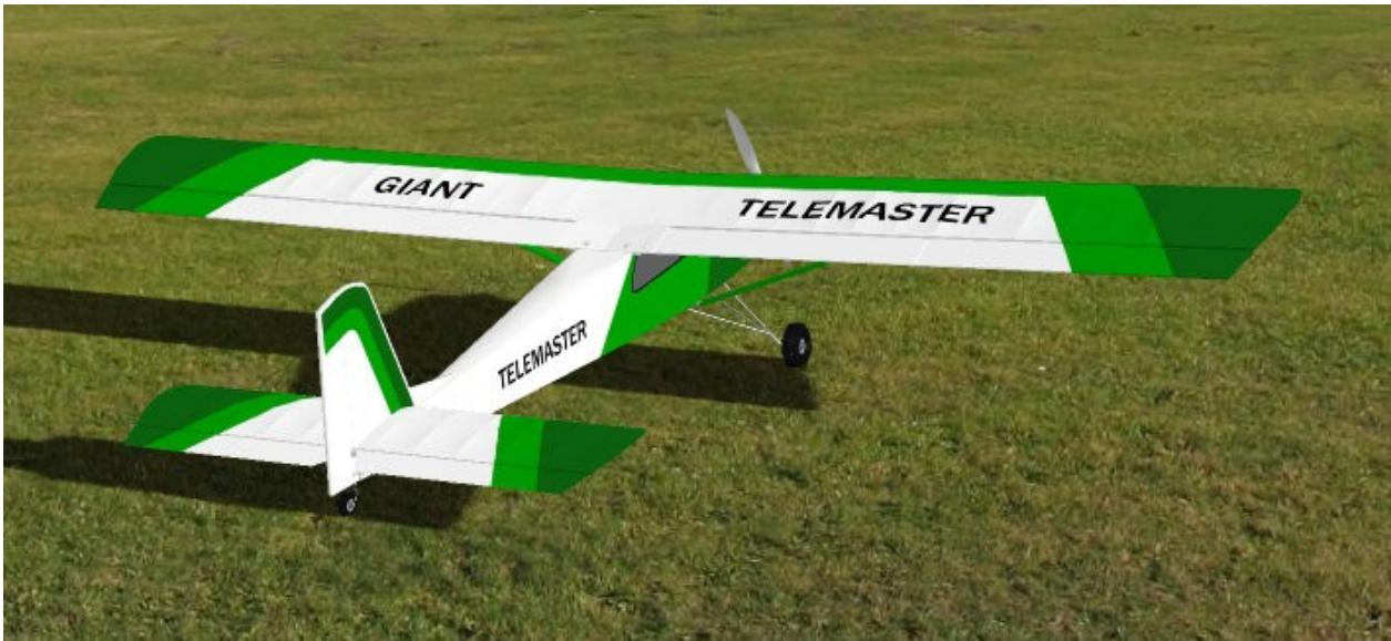
The most obvious differences to the Senior were incorporated into the visual model. The wing dihedral is reduced and lift struts are added. The aluminum plate landing gear was replaced by a wire landing gear, which is lightweight but still able to carry the airframe's weight. Ailerons and flaps are enlarged to 25% of the wing's chord length (instead of 15% on the Senior). There is no flaperon version.
